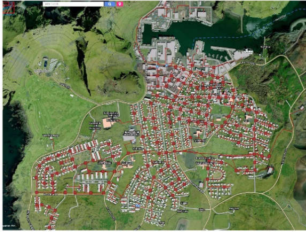
Figure 17, Geothermal distribution network in the small town of Heimaey in Iceland, district heating based on GE found in the preceding local lava eruption, clever method of attaining benefits from a disaster. Iceland is one of the most potent countries with GE, source: www.verkis.is , presentation by T. Johannesson, Cornell University, November 2016, courtesy of the presenter
